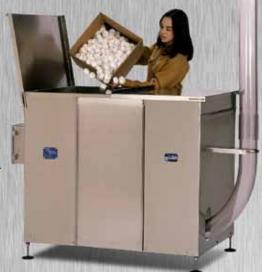
from the unit. PPFs are produced in several sizes using stainless steel construction on all surfaces in contact with the product. With its sturdy construction and simple design, maintenance is as simple as changing filters.
